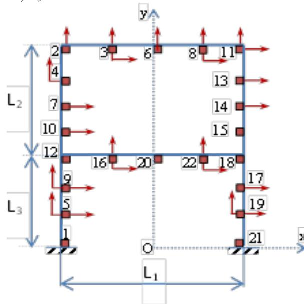
Figure 1: 2D frame ( → Positions of  $c = 24$  sensors)
