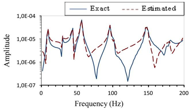
Figure 3:  $p = 4$  optimal selected excitation points, with a modal damping factor  $a_i = 0.01$
