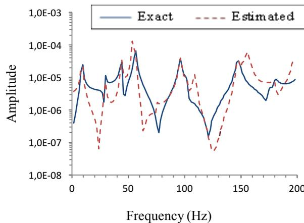
**Figure 2:**  $p=4$  arbitrarily selected excitation points, with a modal damping factor  $a_i = 0.01$
