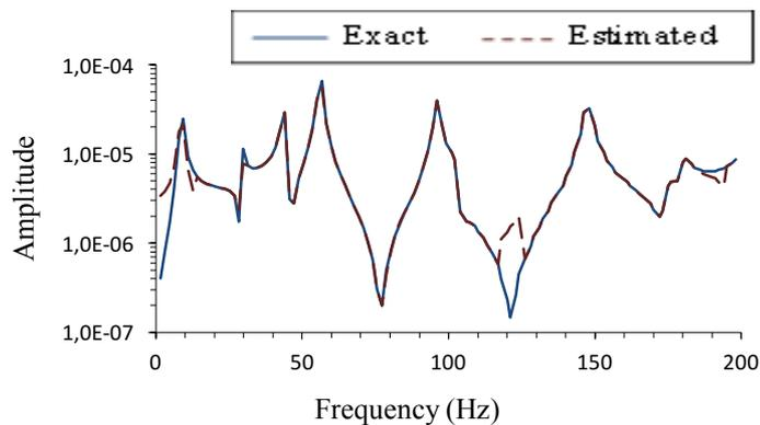
Figure 5:  $p = 8$  optimal selected excitation points, with a modal damping factor  $a_i = 0.01$ , using eq. (25)
